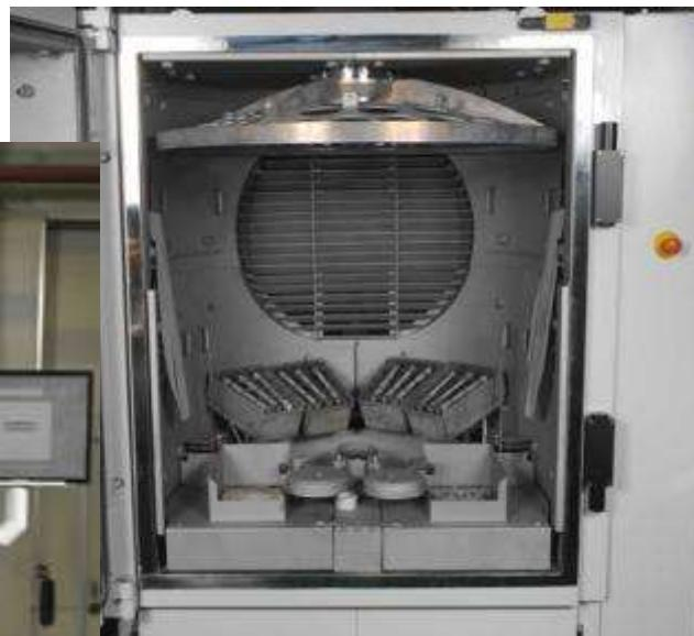
Korea Vac Tec's VTC-1000 PO Coater is designed for precise optical coatings on optical parts and similar products using electron-beam and thermal evaporation (with ion gun pre-cleaning and assistance) to create multilayer optical coating on the surface of substrates. VTC-1000 PO Coater runs in fully automatic mode.
