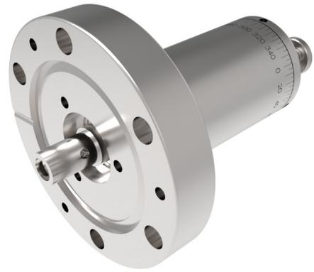
The MD40N MagiDrive provides low torque rotation (0.45Nm) on a 70mm OD (2¾" OD CF) flange. The MD40A MagiDrive provides medium torque rotation (1.8Nm). The drive is ideally suited to applications such as the rotation of samples and small platens, where stability is key.
