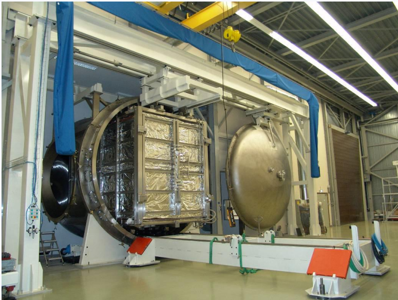
Thermal vacuum chamber (TVC) using 2 sets VELCO 1000
