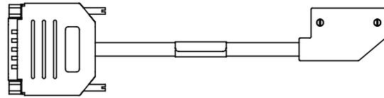
A range of low profile adapter cables have been developed to support replacing older generation MFC's with different pinout configurations. The base MFC will be either a G1, TX or SX configuration, depending on the product being replaced.
