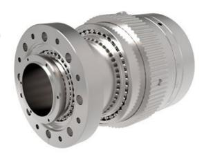
The MD64LB & MD64LBM MagiDrives provides high (8 Nm) or ultra-high (40 Nm) torque rotation through a high stiffness coupling with a large 48.5mm clear bore. This drive is ideally suited to platen rotation or robot type applications. The MD64LBM supplies higher torque with the same dimensions.
